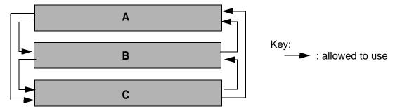
Figures like the one above are why layers have been a source of ambiguity for so long, for architects have been calling such things layered when they are not. There is more to layers than the ability to draw separate parts on top of each other.
