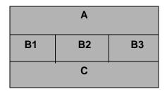
Thick edges. Sometimes the rectangles in a stack are shown with thick horizontal edges denoting the interface to the layer. This is intended to convey the restriction that inter-layer usage only occurs via interface facilities, and not directly to any layer's "internals."
